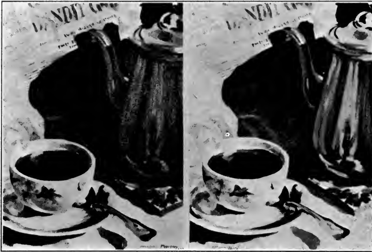
FIG. 8. Oil painting photographed with and without the Pola-screen over lens and lights, crossed. The position of the lights was unchanged. Note the absence of speckle from the canvas ribbing and the great improvement in shadow detail.
